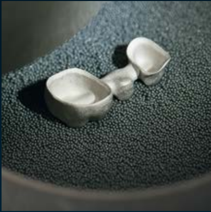
7 Ceramill Sintron® restoration after sintering and removal from the Ceramill Argothem sintering furnace
